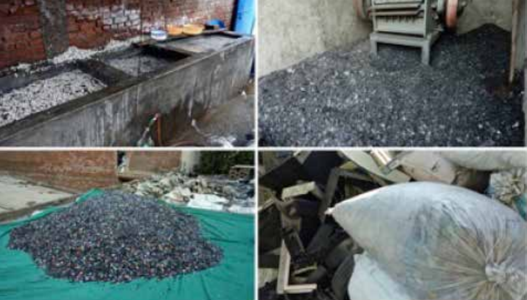
Figure 10. Grinding, float separation and sorting by informal recyclers, India.
