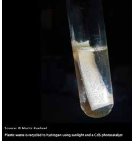
Figure 22. Photoreformation of plastic waste to hydrogen.
