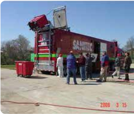
Figure 40a. Sanitech medical waste disinfection system as truck mounted and stationary units.
