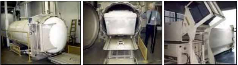
Figure 39. L-R: Bondtech autoclave, on-site autoclave with lift table at a hospital, waste dumper.
