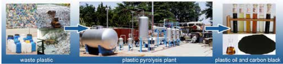
Figure 20. Plastic to fossil fuel via pyrolysis.
